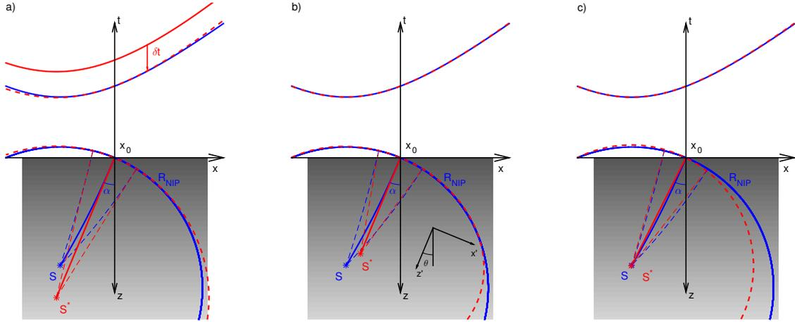
**Figure 1:** NIP experiment in the inhomogeneous medium (blue rays and wavefronts) and its interpretation by optical (a), anisotropic (b) and effective (c) auxiliary media. Note that in the effective medium (c) the actual and image sources do not generally coincide.
