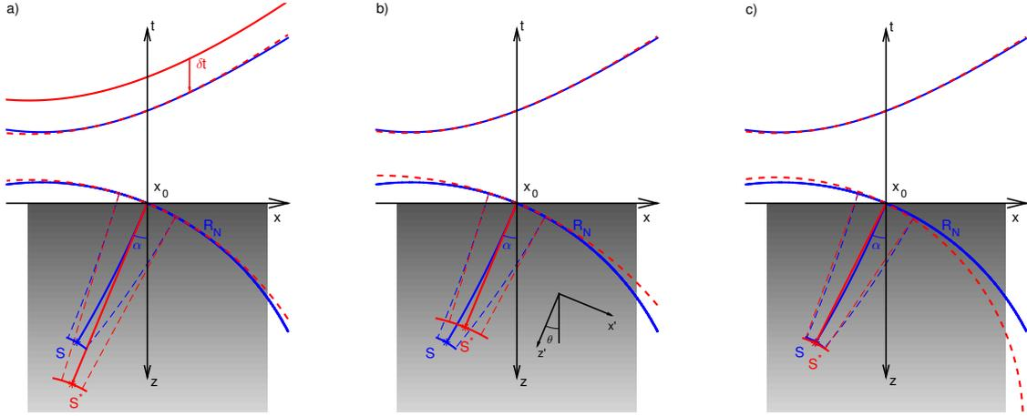
**Figure 2:** Normal experiment in the inhomogeneous medium (blue rays and wavefronts) and its interpretation by optical (a), anisotropic (b) and effective (c) auxiliary media.
