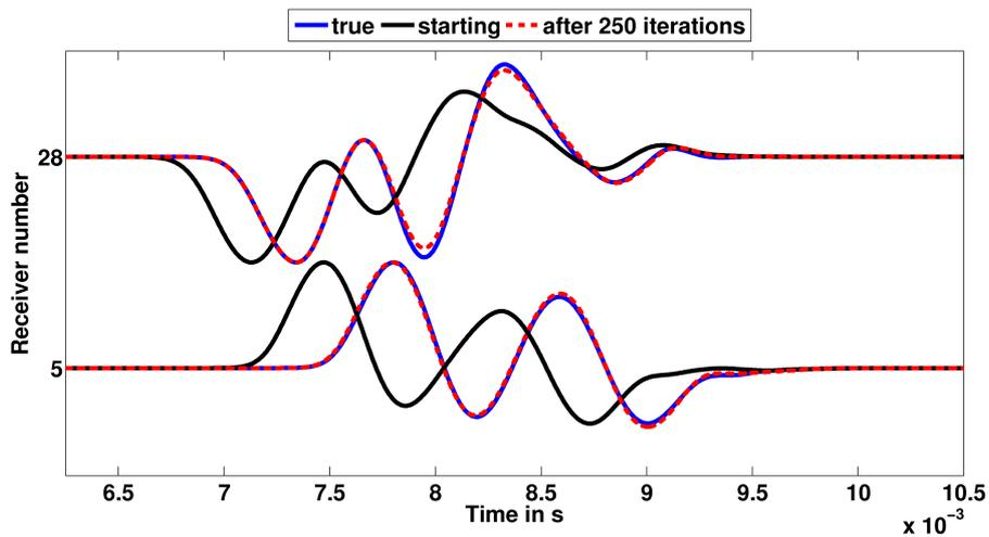
**Figure 5:** Comparison of true (blue), starting (black) and inverted seismograms (red dashed) for receiver 5 and 28 of shot 40.
