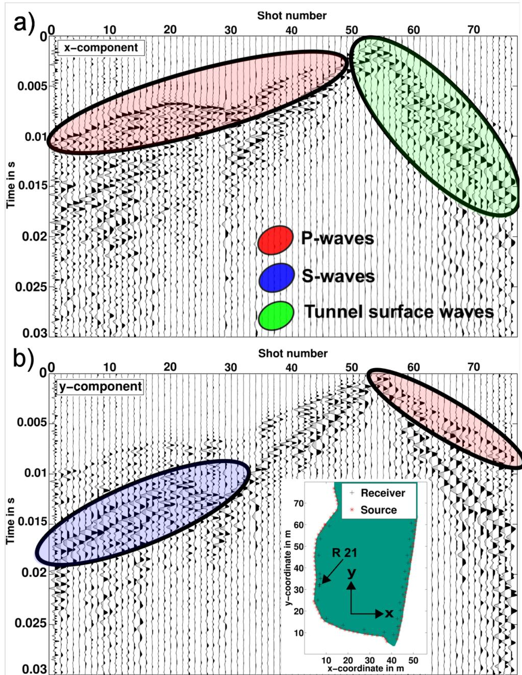
**Figure 2:** Field data: common receiver gather (R 21) of vibroseis data: Traces are normalized to their maximum amplitude. In **a)**, the x-components and in **b)**, the y-component is shown. Different wave types are highlighted with different colors.
