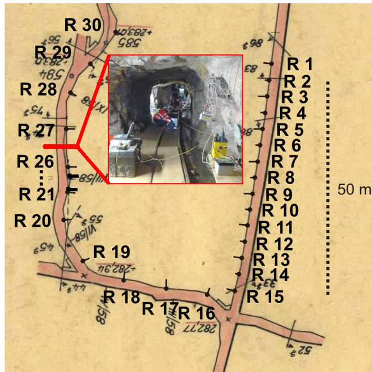
**Figure 1:** Section of an old underground map from the year 1962 showing the measuring area modified after Koop (1962): The block is surrounded by three galleries in a depth of 150 m. 30 3-C receiver anchors are mounted within the block (R 1 to R 30). The photo shows the inside of the left gallery (Photo: A. Jurczyk, GFZ).
