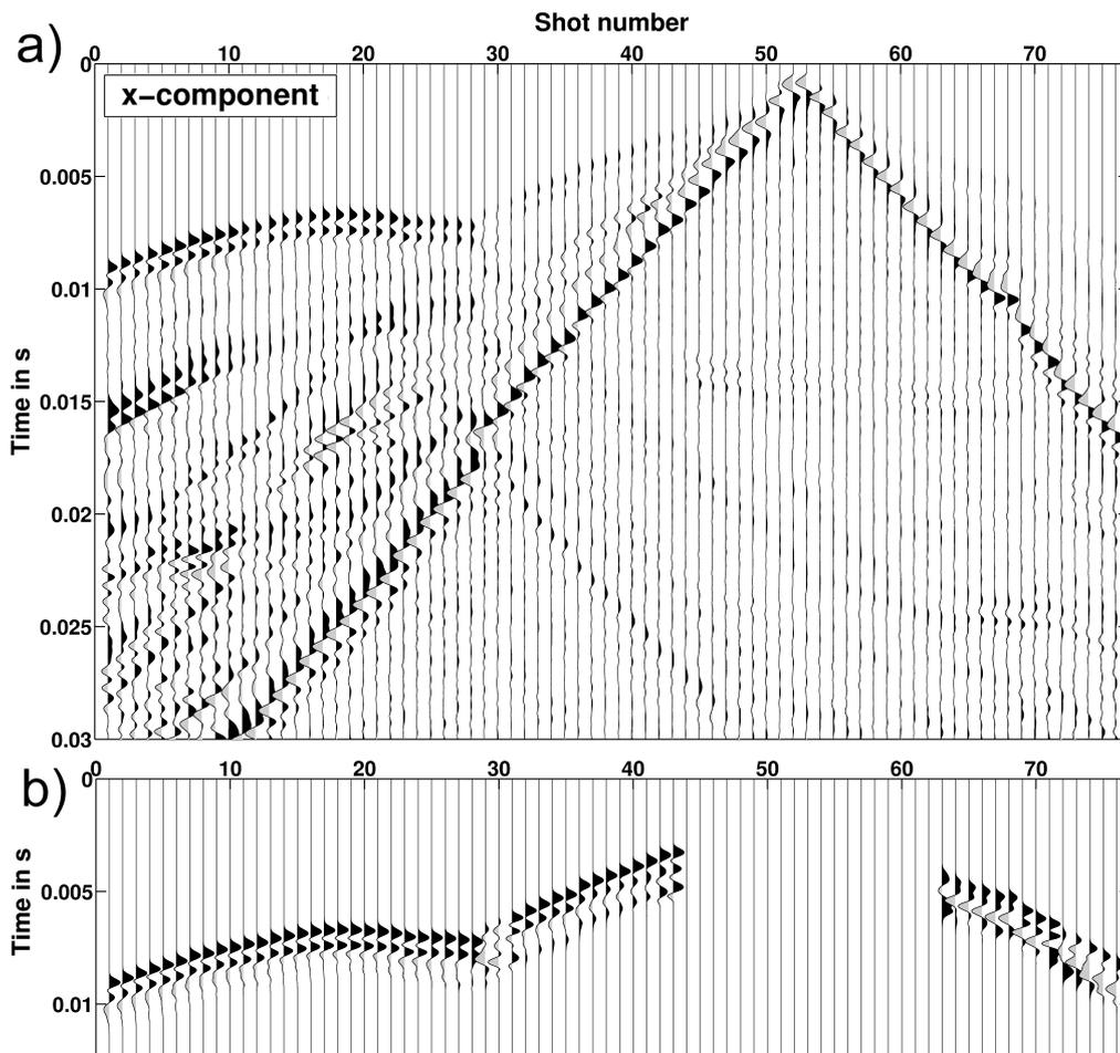
**Figure 3:** Synthetic common receiver gather of receiver 21: The geometry of the sources has been adapted from the field measurement. **a)**, unprocessed seismograms. **b)**, preprocessed data of a).
