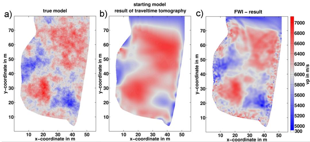
**Figure 4:** Result of synthetic study: **a)** True model: A Random media model with a velocity perturbation which simulates a crystalline rock. **b)** Starting model: The starting  $v_p$  velocity model for the inversion which was derived from a first arrival travel time tomography of the true model. **c)** FWI-result: Inverted  $v_p$  velocity model after 250 iterations using the first arrival P-waves only.
