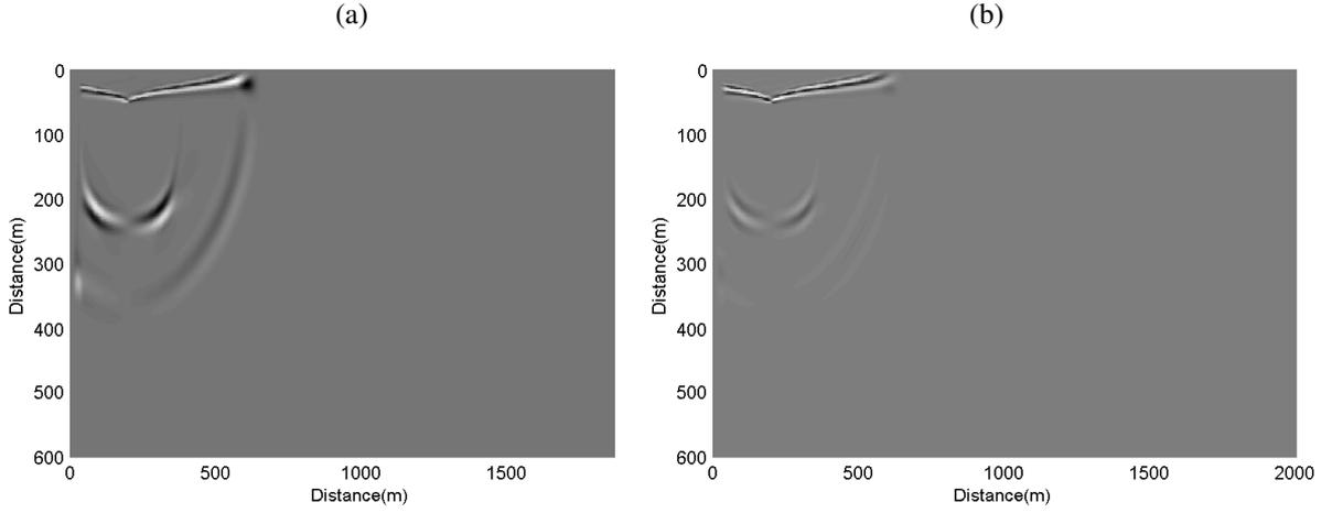
**Figure 4:** Wavefields after applying the (a) curl operator and (b) operator (52) to the snapshots  $u_1$  and  $u_3$  in Figure 2. The curl operator fails to completely separate P and S wavefields for the direct wave, whereas our provides a much better result.
