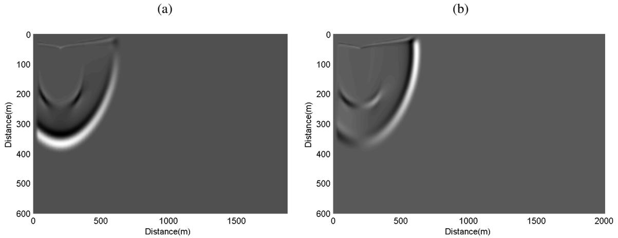
**Figure 2:** 2D snapshots for (a)  $u_1$  and (b)  $u_3$  in a VTI homogeneous medium with  $\epsilon = -0.2187$  and  $\delta = -0.2704$ . We can observe the coupling between  $P$  and  $S$  waves.
