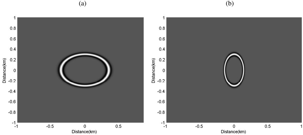
**Figure 1:** 2D snapshots of potential  $\psi$  in the elliptic case, for a point source located at the origin with  $\alpha = 1.5 \text{ km/s}$ : (a)  $\epsilon = \delta = 0.2$ ; (b)  $\epsilon = \delta = -0.39$ .
