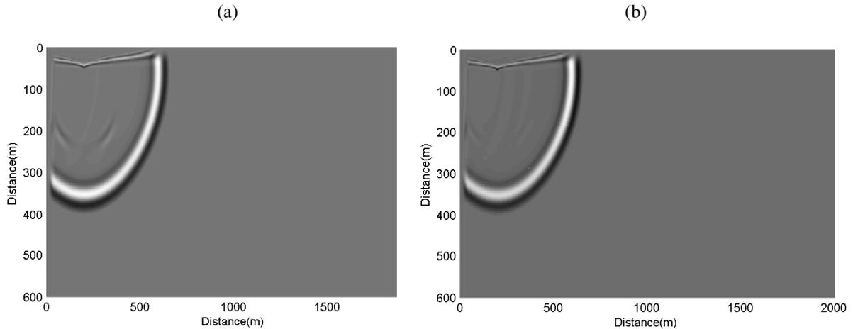
**Figure 3:** Wavefields after applying the (a) divergence operator and (b) operator (46) to the snapshots  $u_1$  and  $u_3$  in Figure 2. We can observe a better suppression of the  $S$  wave for the operator given by (46).
