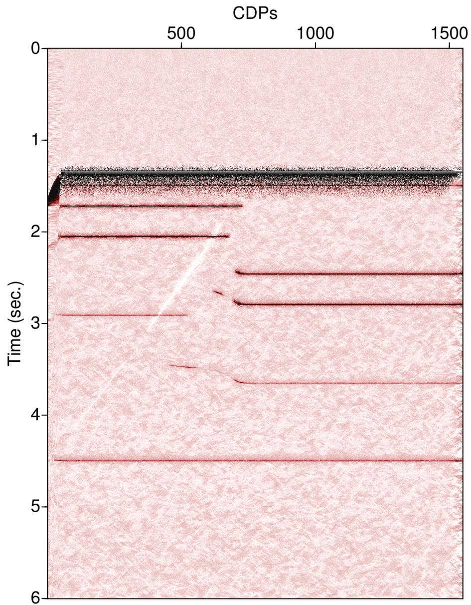
**Figure 3:** CRS stack result for the synthetic data set, without smoothing of  $\beta_0$  and  $K_{NIP}$  sections.
