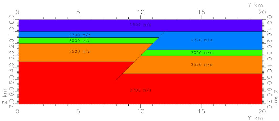
**Figure 2:** Velocity profile of the synthetic model.
