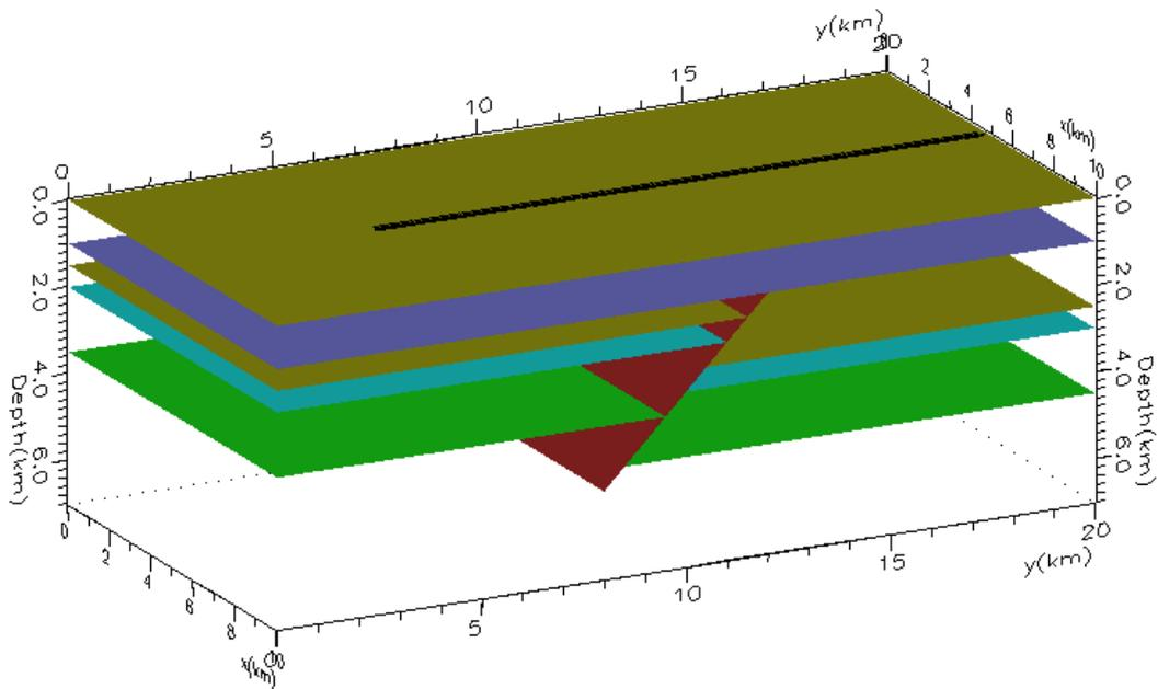
**Figure 1:** 2.5D model used to generate the synthetic data. Acquisition line is highlighted in black.
