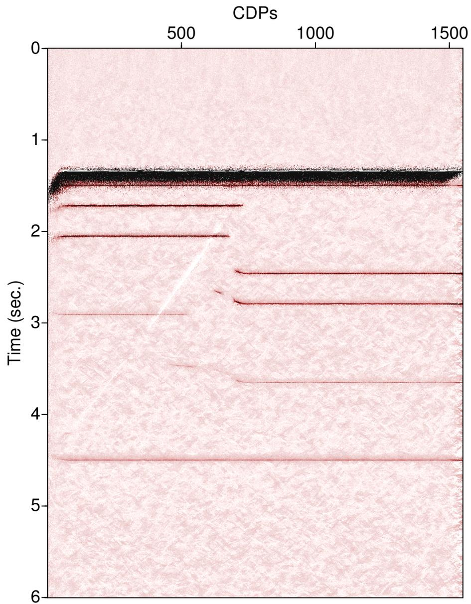
**Figure 4:** CRS stack result for the synthetic data set, with smoothed  $\beta_0$  and  $K_{NIP}$  parameters.
