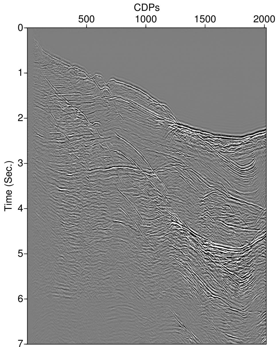
**Figure 5:** CRS stack result for the real marine data set without smoothing of CRS parameters.
