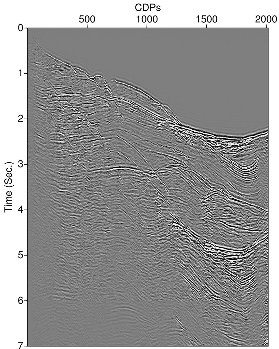
**Figure 6:** CRS stack result for the real marine data set with smoothed CRS parameters  $\beta_0$  and  $K_{NIP}$ .
