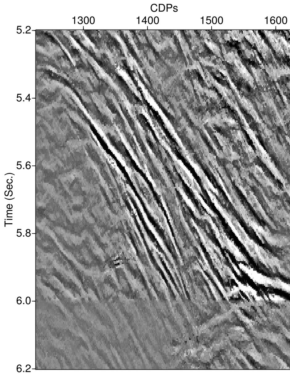
**Figure 7:** Detail from the CRS stack result for the real marine data set without parameter smoothing.
