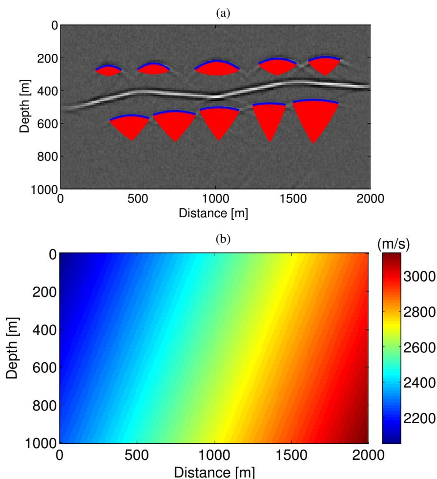
**Figure 6:** (a) Remigration trajectories collapsing in the depth point where depth migration should be located if the correct velocity model had been used. (b) The average velocity model from interpolation of velocity values at each diffraction point.
