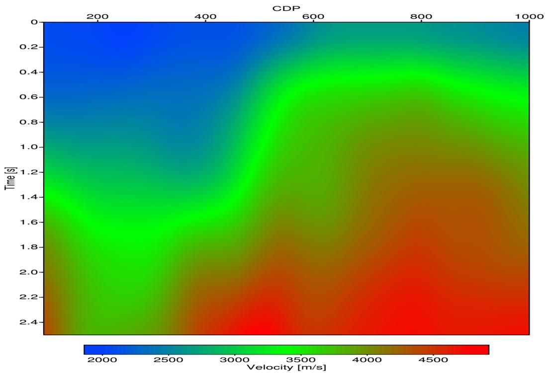
**Figure 2:** Stacking Velocity model resulting from the conventional processing.
