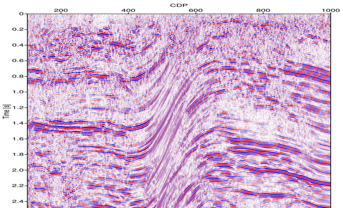
**Figure 4:** ZO stacked section obtained by the one-step CRS stack without using the stacking velocity.
