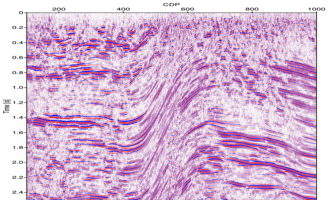
**Figure 5:** ZO stacked section obtained by the multi-step CRS stack using the stacking velocity.
