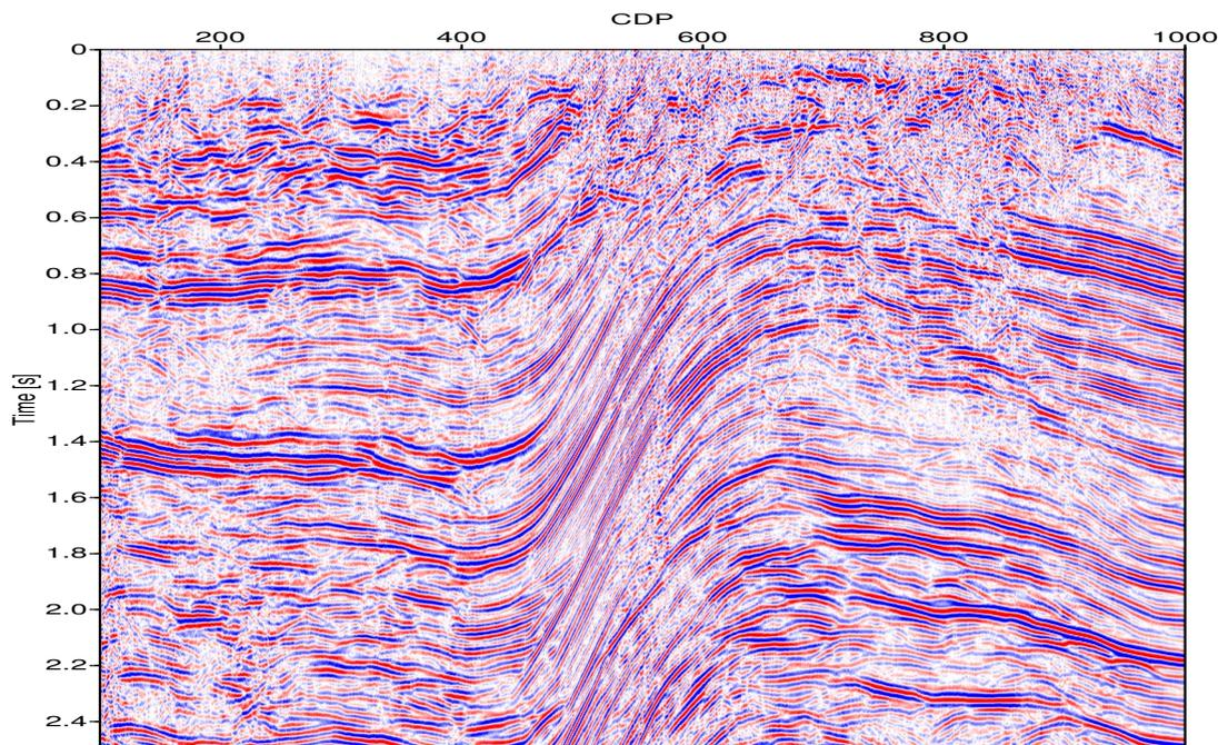
**Figure 6:** ZO stacked section obtained by the one-step CRS stack using the stacking velocity.
