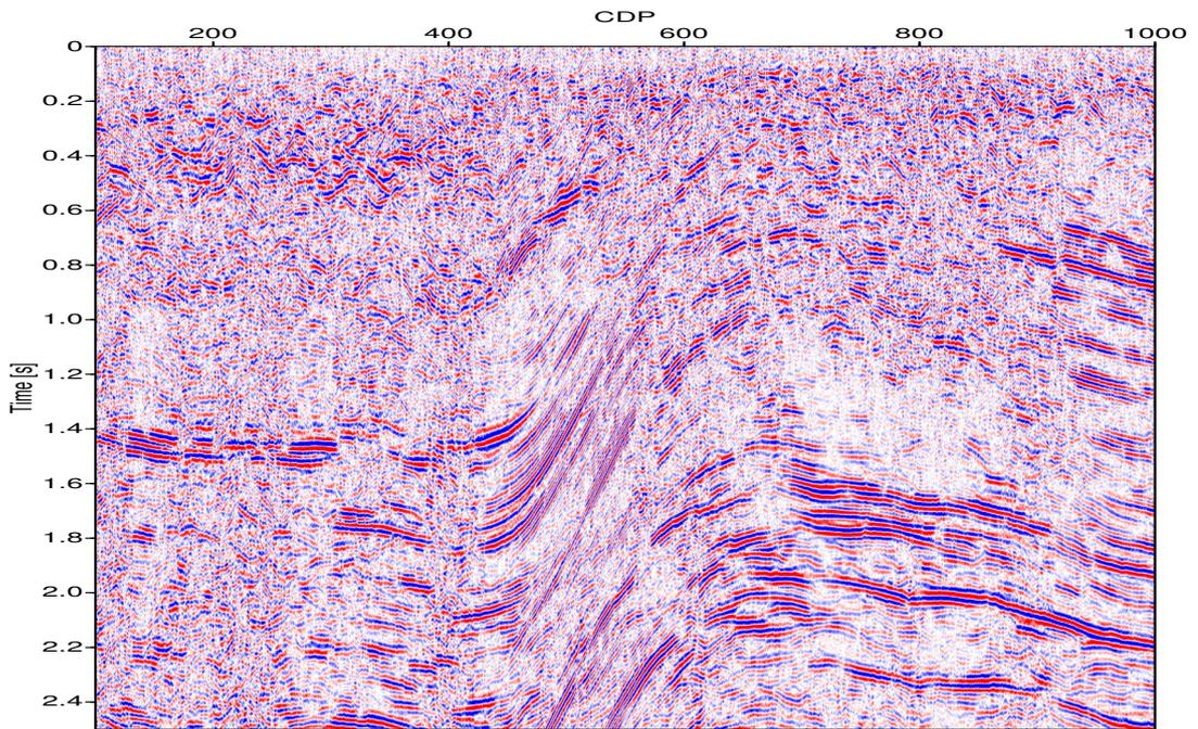
**Figure 3:** ZO stacked section obtained by the multi-step CRS stack without using the stacking velocity.
