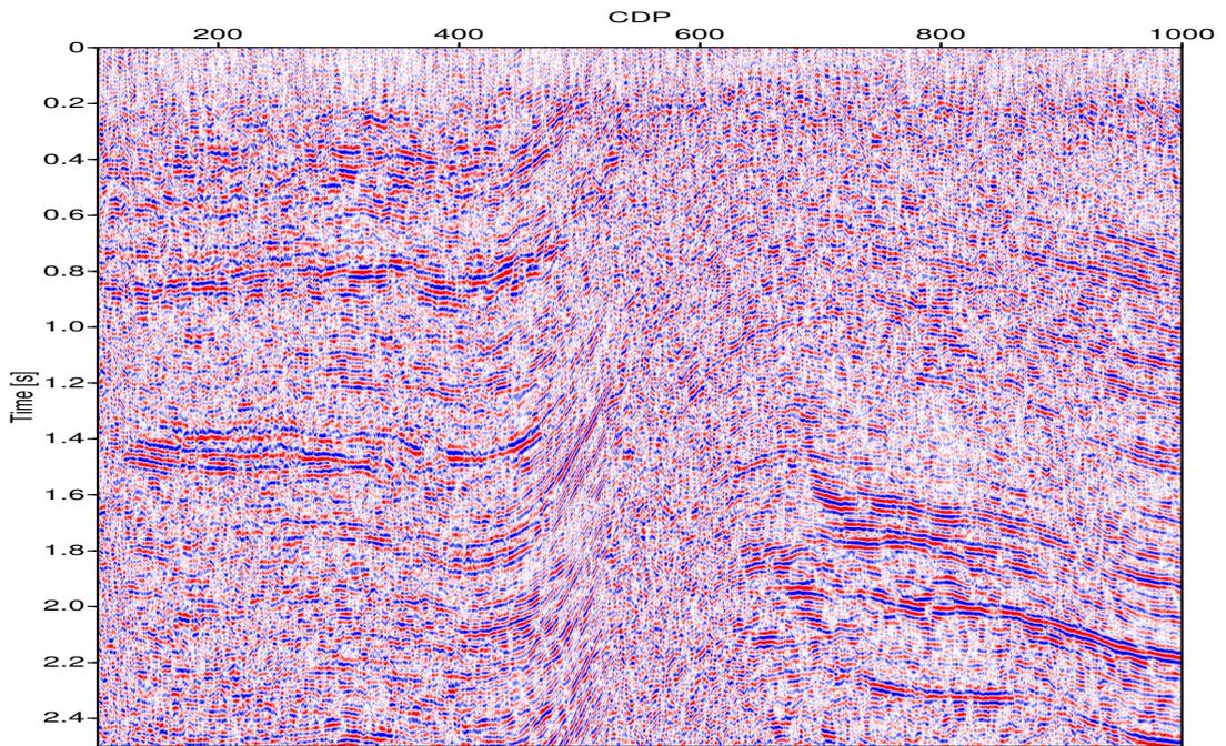
**Figure 1:** ZO stacked section obtained by the CMP (NMO/DMO) stack method.
