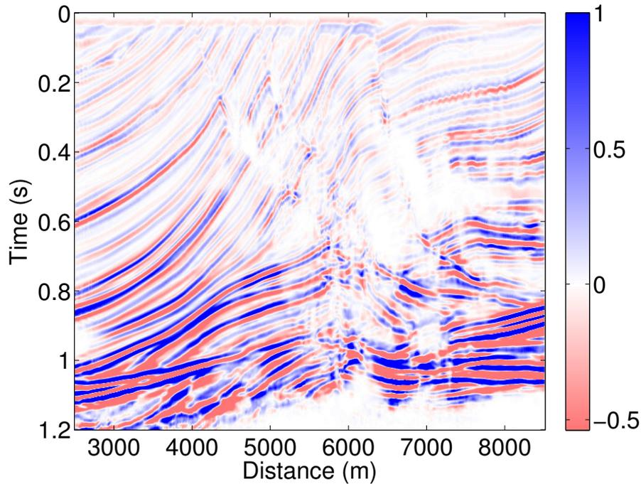
**Figure 2:** Result of multipath-summation time imaging.
