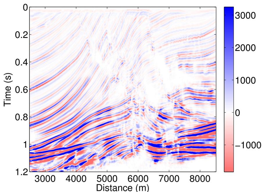
**Figure 3:** Result of multipath-summation time imaging with additional velocity weight.
