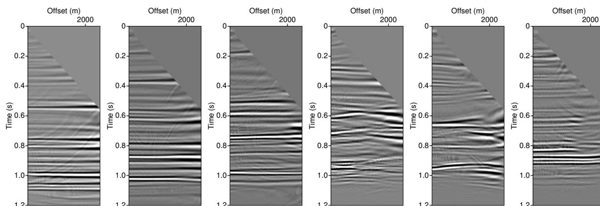
**Figure 14:** Common-image gathers from time migration using velocities extracted by masked division plus moving-average smoothing.
