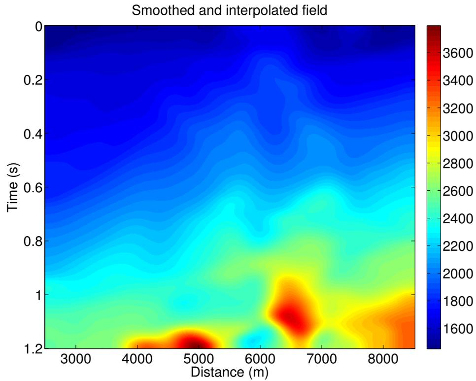
**Figure 10:** Velocities extracted by masked division plus moving-average smoothing.
