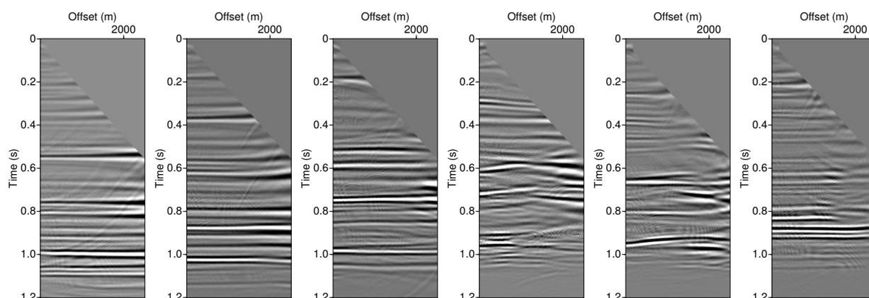
**Figure 15:** Common-image gathers from time migration using velocities extracted by masked division plus B-splines smoothing.
