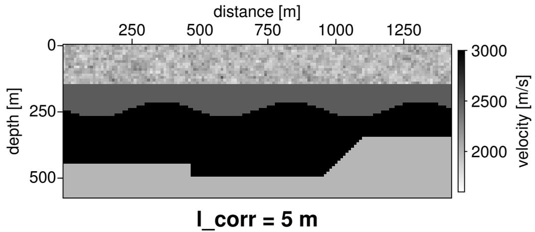
**Figure 5:** Model with a correlation length of 5 m in the surface layer
