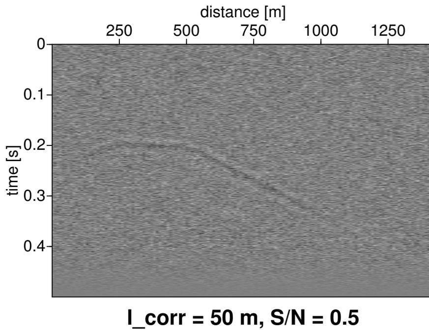
**Figure 13:** Seismogram section from model in Fig. 11 with noise added. Signal to noise ratio is 0.5
