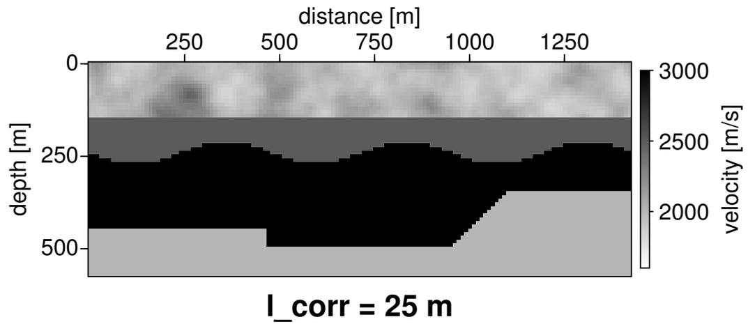
**Figure 9:** Model with a correlation length of 25 m in the surface layer
