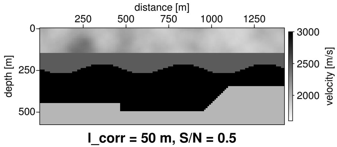
**Figure 11:** Model with a correlation length of 50 m in the surface layer
