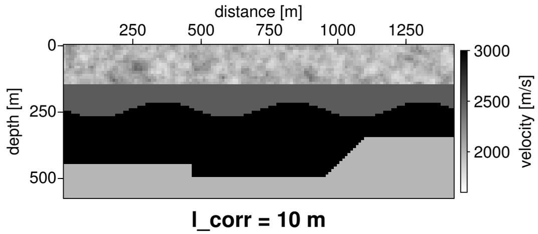
Figure 7: Model with a correlation length of 10 m in the surface layer
