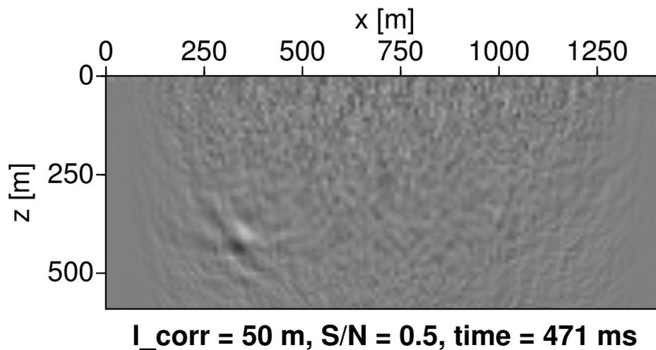
**Figure 14:** Snapshot at source time estimated from reverse modelling of seismogram recordings in Fig. 13.
