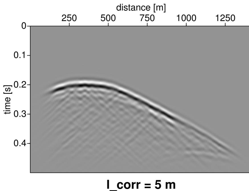
**Figure 6:** Seismogram section from model in Fig. 5
