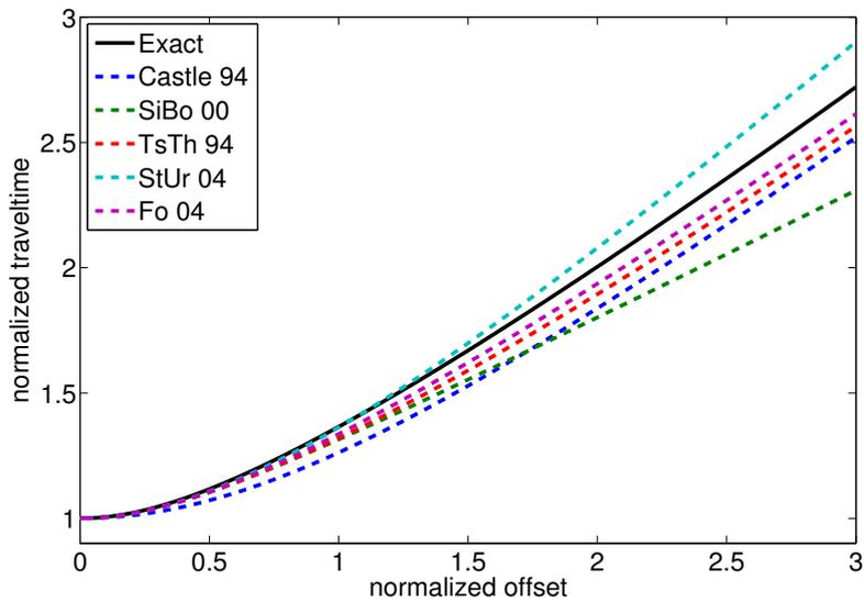
**Figure 2:** Comparison of traveltime approximations (4) (shifted hyperbola) with  $S = S(x)$  [Castle 94] and  $S = 1 + 8\eta$  [SiBo 00], (6) [TsTh 94], (7) [StUr 04], and (10) [Fo 04] with the exact VTI traveltime.
