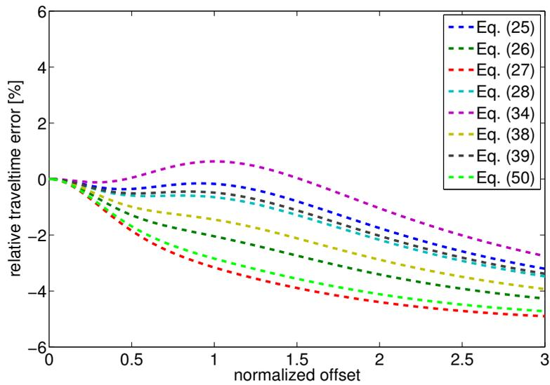
**Figure 7:** Relative error of new traveltime approximations for  $t(x)$  of the type  $t(x) \approx t_h(x) + B(\eta) \frac{x^2}{t_h^3(x)}$ .
