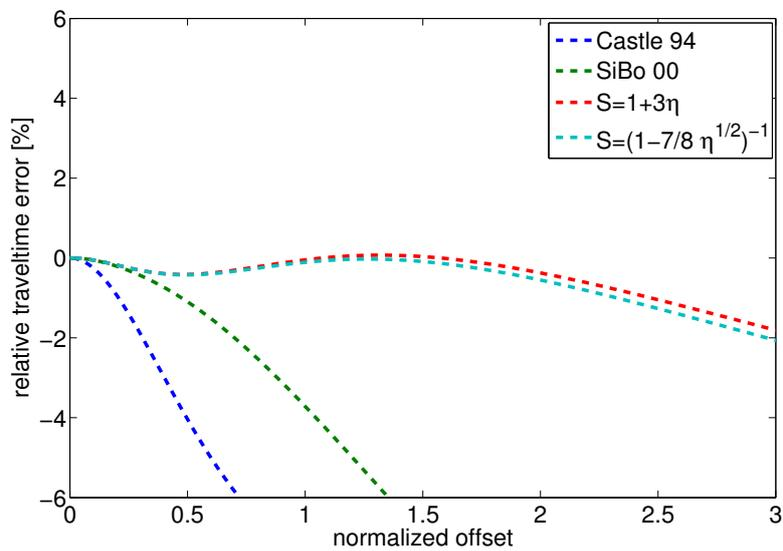
**Figure 9:** Relative error of shifted hyperbola with  $S = S(x)$  [Castle 94],  $S = 1 + 8\eta$  [SiBo 00], and new shifted hyperbola approximations with  $S = 1 + 3\eta$  and  $S = \left(1 - \frac{7}{8}\sqrt{\eta}\right)^{-1}$ .
