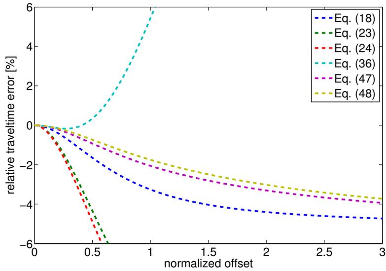
**Figure 6:** Relative error of other traveltime approximations for  $t^2(x)$ .
