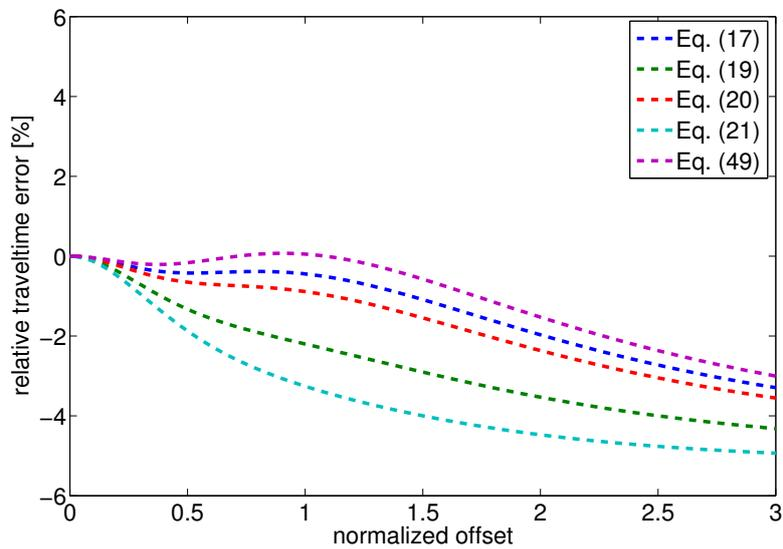
**Figure 5:** Relative error of new traveltime approximations for  $t^2(x)$  of the type  $t^2(x) = t_h^2(x) + B(\eta) \frac{x^2}{t_h^2(x)}$ .
