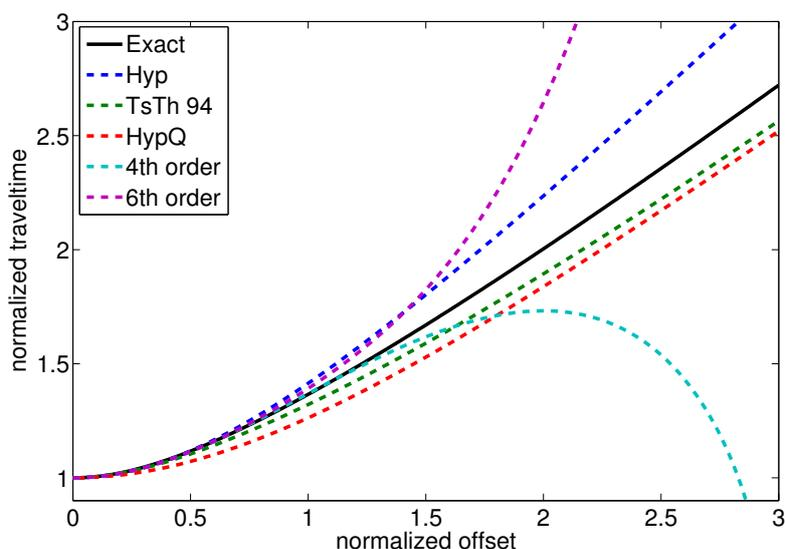
**Figure 1:** Comparison of traveltime approximations (1) [Hyp], (6) [TsTh 94], (11) [HypQ], as well as the 4th order and 6th order approximations of Bolshix (1956) with the exact VTI traveltime.
