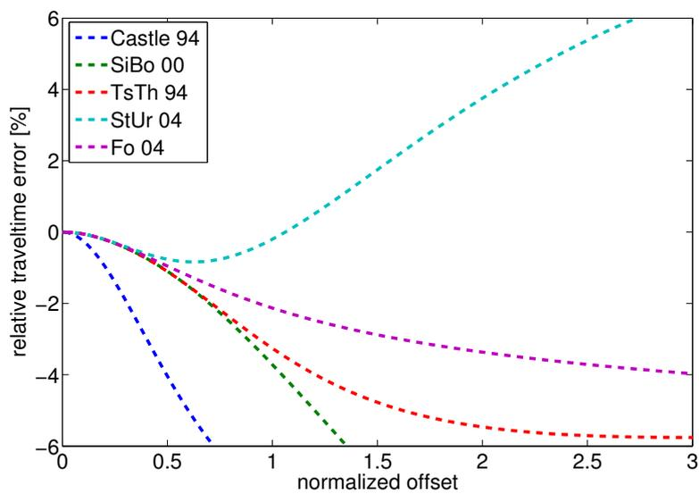
**Figure 3:** Relative error of traveltime approximations (4) (shifted hyperbola) with  $S = S(x)$  [Castle 94] and  $S = 1 + 8\eta$  [SiBo 00], (6) [TsTh 94], (7) [StUr 04], and (10) [Fo 04].
