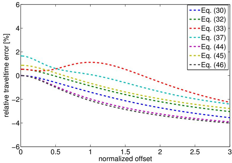
**Figure 8:** Relative error of other traveltime approximations for  $t(x)$ .
