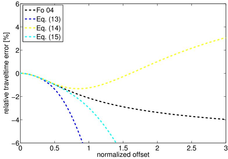
**Figure 4:** Relative error of traveltime approximation (10) [Fo 04] and its Padé approximations [2,2], [4,2] and [4,4].
