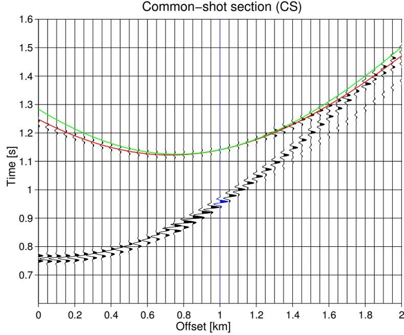
**Figure 7:** CS section: The red line corresponds to the traveltime calculated with equation (6) and the green line corresponds to the traveltime calculated with equation (7).
