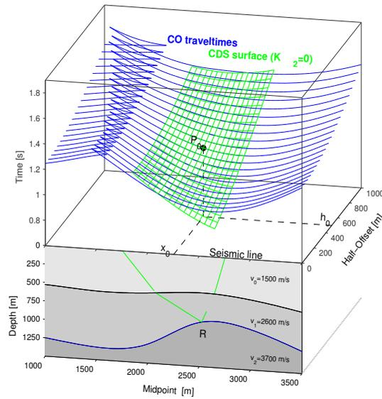
**Figure 11:** Lower part (front): 2D media with three homogeneous layers separated by curved and smooth interfaces and a FO central ray, where  $x_0$  is the midpoint,  $h_0$  is the half-offset. Upper part: CO traveltimes curves (blue color) related to primary reflections of the second interface with the CDS operator when  $K_2 = 0$  (green color), associate to  $P_0$ .
