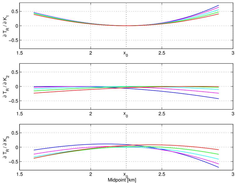
**Figure 10:** Sensibility through FO CRS traveltimes derivative with respect  $K_1$  (top),  $K_2$  (middle) and  $K_3$  (bottom) for different offsets,  $h = 0.0\text{km}$  (blue curve),  $h = 0.25\text{km}$  (magenta curve),  $h = 0.5\text{km}$  (cyan curve),  $h = 0.75\text{km}$  (green curve) and  $h = 1.0\text{km}$  (red curve).
