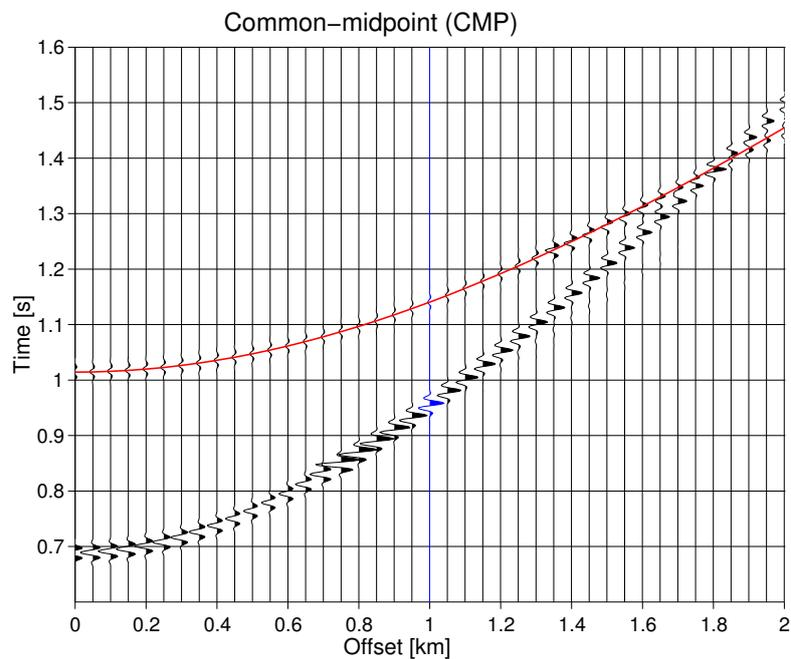
**Figure 5:** CMP section corresponding for the midpoint 2250 m. The red line corresponds to the traveltimes calculated with equation (3) for the second reflector. For this configuration, the traveltimes curve is the same for reflection and diffraction events.
