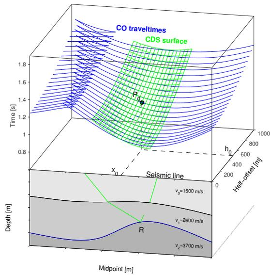
**Figure 4:** Lower part (front): 2D media with three homogeneous layers separated by curved and smooth interfaces and a FO central ray, where  $x_0$  is the midpoint,  $h_0$  is the half-offset. Upper part: CO traveltimes curves (blue color) related to primary reflections of the second interface with the CDS operator (green color), associate to  $P_0$ .
