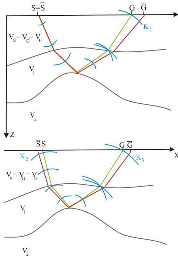
**Figure 2:** 2-D model of three homogeneous layers separated by curved and smooth interfaces: (a) Propagation of the wavefront of the CS experiment at different instants of time, (b) Propagation of hypothetical wavefronts of a CMP experiment at different instants of time.
