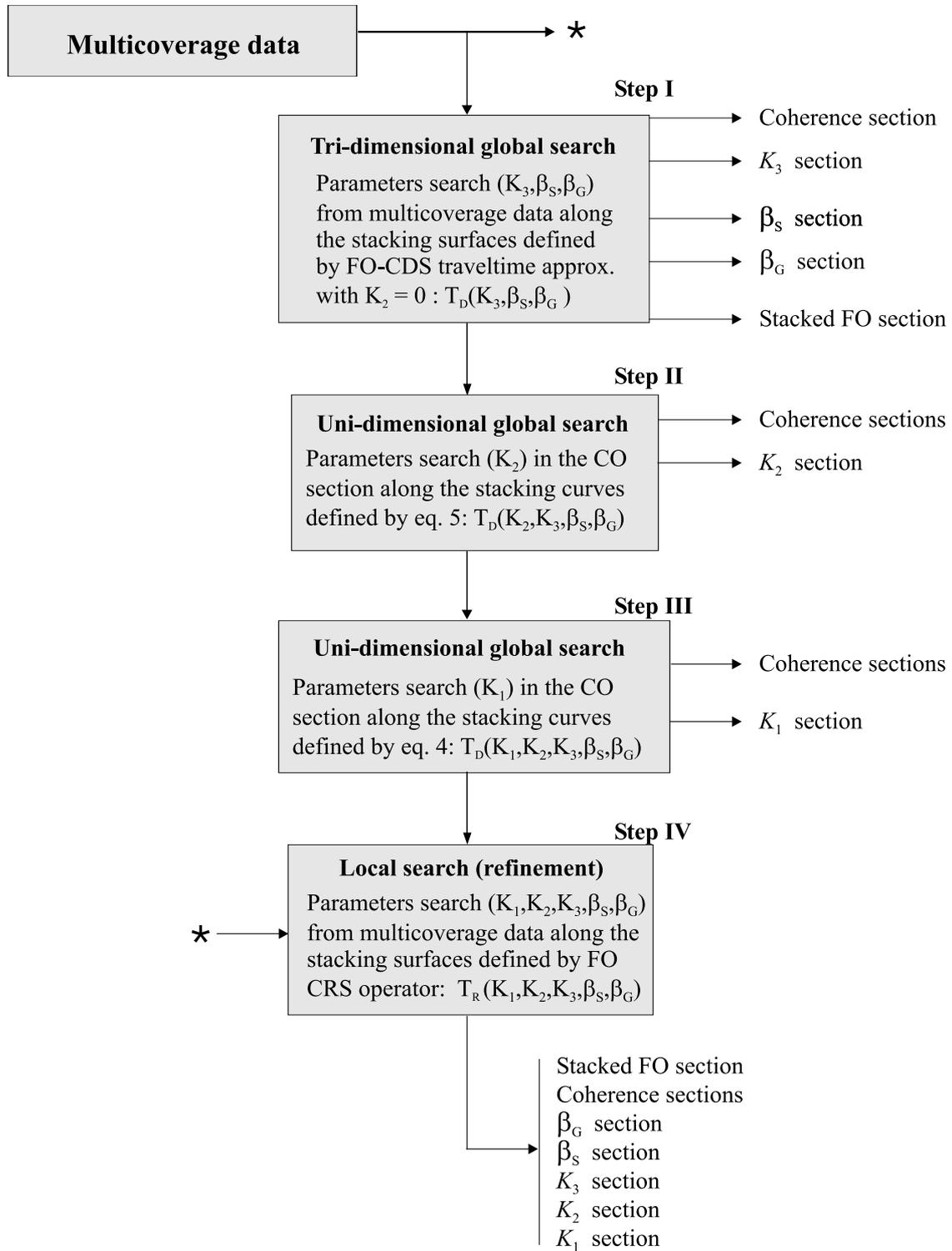
Figure 12: Flowchart of the CO-CRS stacking algorithm.
