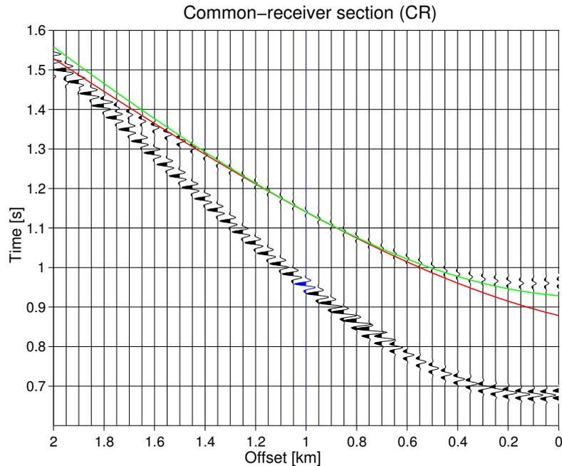
**Figure 8:** CR section. The red line corresponds to the traveltimes calculated with equation (8) and green lines correspond the traveltimes calculated with equation (9).
