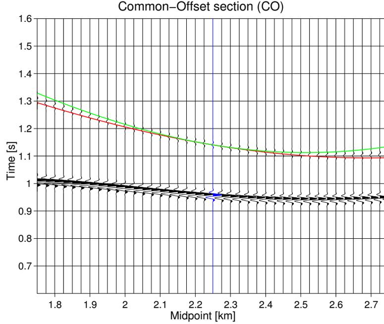
**Figure 6:** CO section which offset is 1 km. The red line corresponds to the traveltimes calculated with equation (4) and the green line corresponds to the traveltimes calculated with equation (5).
