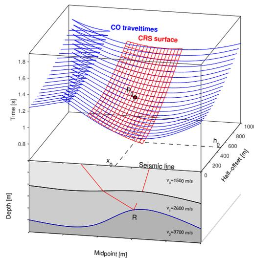
**Figure 3:** Lower part (front): 2D media with three homogeneous layers separated by homogeneous smooth interfaces and a finite-offset central ray, where  $x_0$  is the midpoint,  $h_0$  is the half-offset. Upper part: CO traveltimes curves (blue color) related to primary reflections of the second interface, having the CRS stacking operator (red color) associated to point  $P_0$ .
