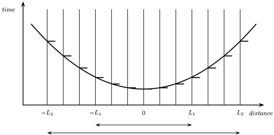
**Figure 1:** Impulse synthetic seismograms of an event with the diffraction traveltime curve for the exact hypocentral time and correct source position. Stacking along this curve provides maximum amplitude. The strength of the amplitude, however, depends on the size of the aperture  $L_1$  or  $L_2$ .
