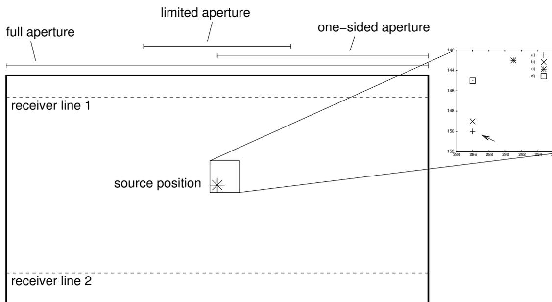
**Figure 3:** Localizations depending on different receiver line apertures. In insert: a) full aperture lines 1 and 2, b) full aperture line 1, c) one-sided aperture line 1, d) symmetric shortened aperture line 1. The arrow shown in the enhanced source region points to the exact source position indicated by a plus sign.
