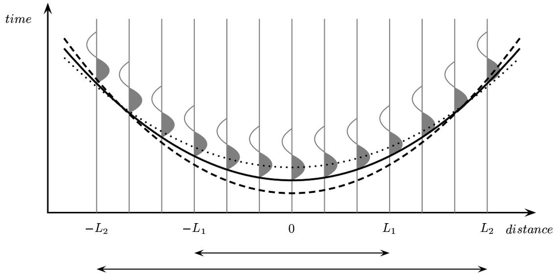
**Figure 2:** Seismic section for the exact hypocentral-time  $t = t_0$  with three traveltimes curves representing sources at the exact location  $(x_0, z_0)$  (solid) and for positions above (dashed) with higher move out and below (dotted) with smaller move out. Details are given in the text.
