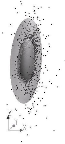
**Figure 4:** The ellipsoids representing different hydraulic diffusivity tensors shown together with the seismic cloud in the scaled coordinate system:  $r_{si} = \frac{r_i}{\sqrt{4\pi t}}$  looking from the south.
