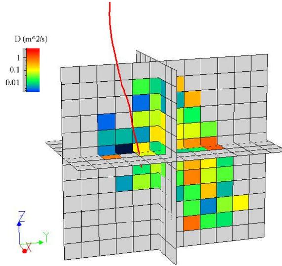
**Figure 5:** Hydraulic diffusivity reconstruction in three dimensions for the Soutz 2000 data set looking from the south-east. The X and Y coordinates represent strikes of N70°E, N340°E, respectively. The diffusivity is given on a logarithmic scale. It varies between 0.001 and 1  $m^2/s$ . A cell has the following spatial dimension  $dx=110$  m,  $dy=130$  m,  $dz=120$  m. The well GPK-2 is also represented in red.
