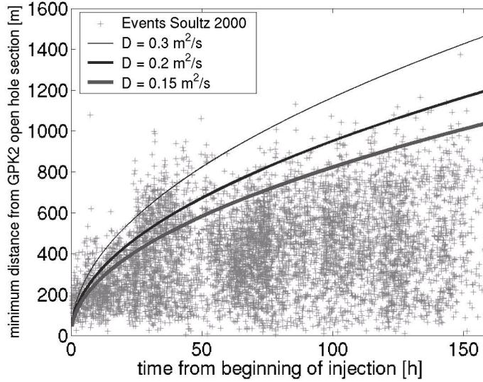
**Figure 3:** r-t plot of the hydraulic stimulation Soultz-2000. Possible estimations of the hydraulic diffusivity are:  $D=0.15 \text{ m}^2/\text{s}$ ,  $D=0.2 \text{ m}^2/\text{s}$ , and  $D=0.3 \text{ m}^2/\text{s}$ . The global estimation,  $D=0.15 \text{ m}^2/\text{s}$ , seems to be more representative.
