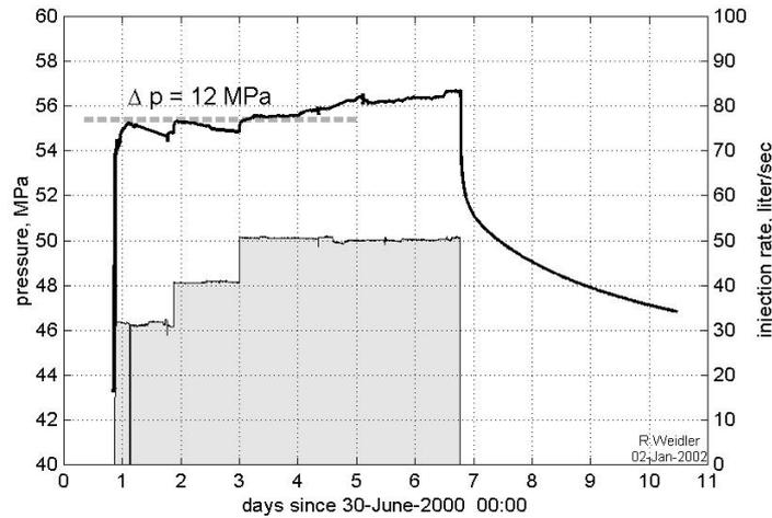
**Figure 1:** Downhole pressure in the open hole section of the well GPK-2 during the hydraulic stimulation Soultz-2000 after Weidler et al.(2002). During the first two injection steps, the maximum overpressure was limited to 12 MPa. During the 50 l/s step, the pressure increased to a maximum value of 13 MPa. These values were still far below the expected values that resulted from an extrapolation of the stress-field in the upper reservoir (3.5 km).
