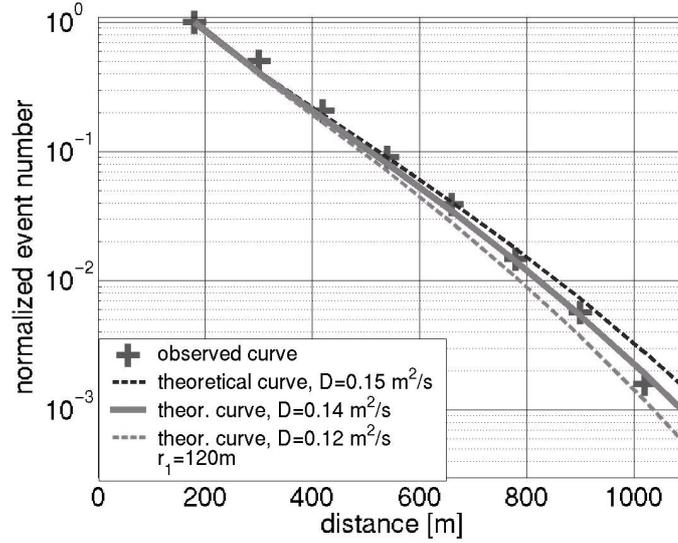
**Figure 6:** Spatial density of the microseismic cloud versus distance from the injection source for the microearthquakes induced during the hydraulic stimulation Soutz-2000. The best fit estimate of the hydraulic diffusivity is  $D=0.14 \text{ m}^2/\text{s}$ . The two dashed curves ( $D=0.12 \text{ m}^2/\text{s}$  and  $D=0.15 \text{ m}^2/\text{s}$ ) illustrate the accuracy of the method.
