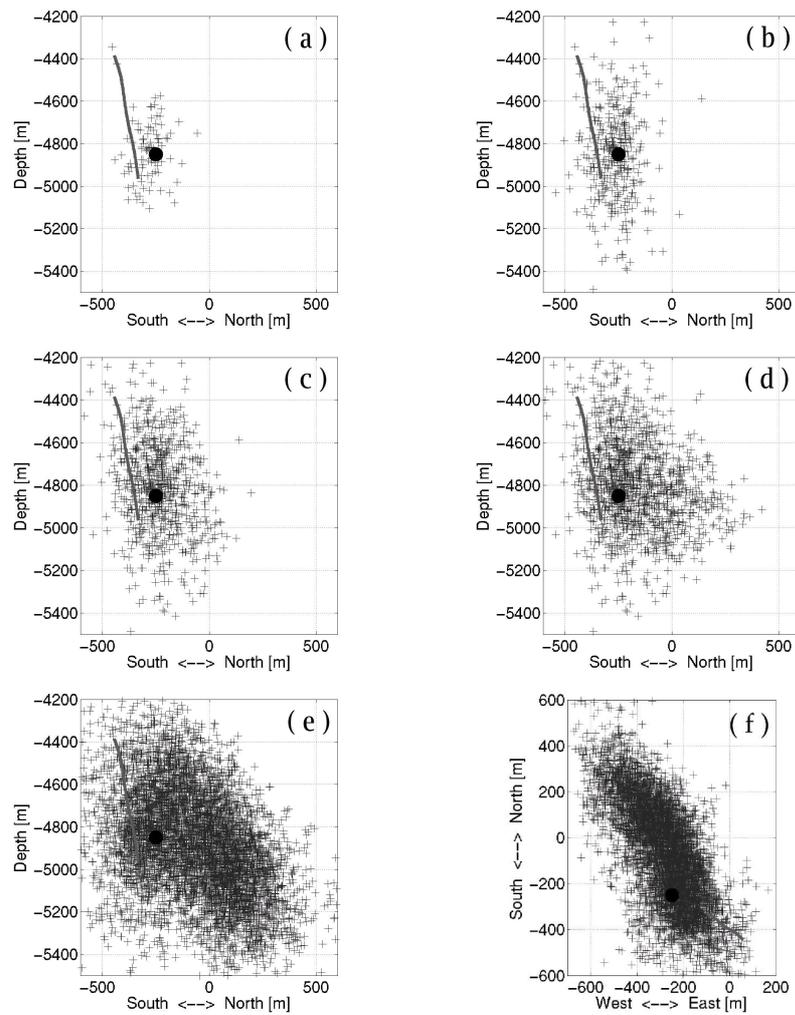
**Figure 2:** Evolution of the cloud of events with time during the hydraulic stimulation Soutz-2000. The line and the black dot denote the open hole section of the well GPK-2 and the point-like source. The snap shots (a),(b),(c),(d) represent the cumulative cloud of events at 3, 10, 20, 30 hours looking from the east. The snap shots (e) and (f) represent the seismic cloud at the end of the injection time ( $t=142.5$  h) from the east and the top respectively.
