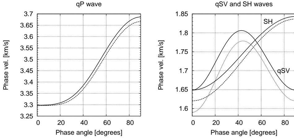
**Figure 4:** Exact and determined phase velocities following from the 21 inverted elastic parameters for the model with 10% anisotropy. Exact phase velocities are displayed by solid lines. Phase velocities computed from the determined parameters are shown by dashed lines for the  $qP$ -wave (left), and by dashed and dotted lines for  $SH$ - and  $qSV$ -waves, respectively (right).
