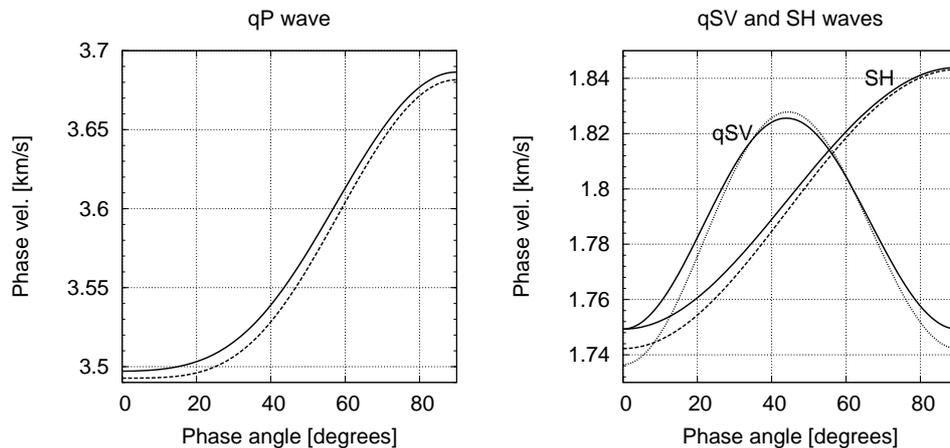
**Figure 7:** Exact and determined phase velocities following from 5 inverted elastic parameters for the model with 5% anisotropy. Exact phase velocities are displayed by solid lines. Phase velocities computed from the determined parameters are shown by dashed lines for the  $qP$ -wave (left), and by dashed and dotted lines for the  $SH$ - and  $qSV$ -waves, respectively (right).
