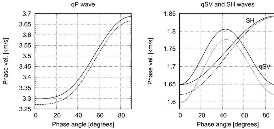
**Figure 5:** Exact and determined phase velocities following from 5 inverted elastic parameters for the model with 10% anisotropy. Exact phase velocities are displayed by solid lines. Phase velocities computed from the determined parameters are shown by dashed lines for the  $qP$ -wave (left), and by dashed and dotted lines for the  $SH$ - and  $qSV$ -waves, respectively (right).
