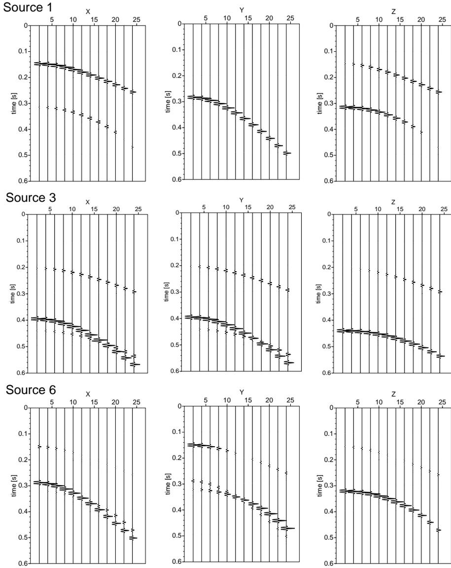
**Figure 2:** Synthetic three-component data for the source positions 1, 3 and 6 (see Fig. 1) for the model with 10% anisotropy. The vertical component is  $Z$  (right), the horizontal components are  $X$  and  $Y$  (left and center). Orientations of  $X$ ,  $Y$  and  $Z$  are along the axis of the general cartesian coordinate system. The traveltime is given on the vertical axis against the receiver number on the horizontal axis. Both split shear waves are visible for the sources at 3 and 6.
