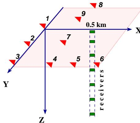
**Figure 1:** The observation scheme of the numerical experiment. A vertical borehole contains 25 aligned three-component receivers with 30 m spacing until a depth of 750 m. The source positions on the surface denoted by reference numbers are indicated by triangles. Sources represent a tilted unit force with fixed orientation for all shots (see eq. 10).
