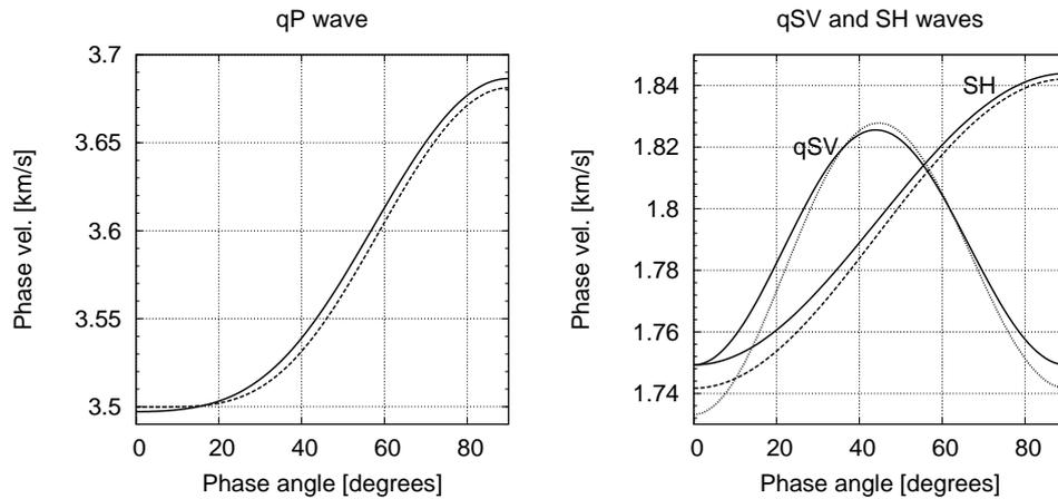
**Figure 6:** Exact and determined phase velocities following from 21 inverted elastic parameters for the model with 5% anisotropy. Exact phase velocities are displayed by solid lines. Phase velocities computed from the determined parameters are shown by dashed lines for the  $qP$ -wave (left), and by dashed and dotted lines for the  $SH$ - and  $qSV$ -waves, respectively (right).
