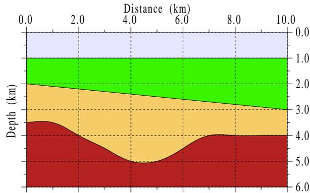
**Figure 5:** Synthetic 2D model with four constant velocity layers.  $v_1 = 2.2$  km/s,  $v_2 = 2.5$  km/s,  $v_3 = 3.0$  km/s, and  $v_4 = 3.5$  km/s from top to bottom.
