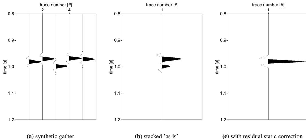
**Figure 2:** Example of residual static correction enhancement after an approximate NMO correction was applied.
