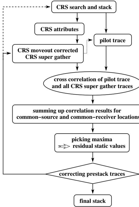
**Figure 4:** Flowchart for the iterative residual static correction by means of CRS attributes. For the second and further iterations, the CRS search for the attributes can be optionally performed again but this will need more processing time. If not, the pilot trace has to be recalculated from the CRS moveout corrected CRS super gather to take advantage of the enhancements of the first or previous iterations.
