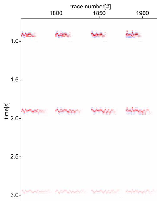
**Figure 7:** This is a part of the CRS moveout corrected CRS super gather for CMP 120. The CMPs within the CRS aperture are shown one after the other and their traces are consecutively numbered. It is obvious that the moveout correction did not correct the random residual statics. The reflection events are more or less flattened.
