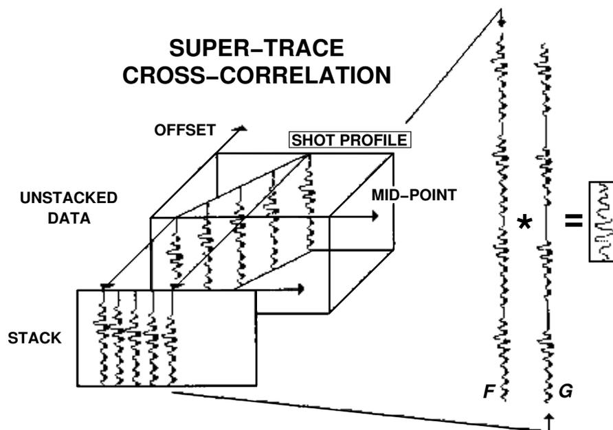
**Figure 3:** Example of super-traces for one moveout corrected shot gather. Super-trace F and super-trace G are cross correlated to determine the corresponding source static. Figure taken from Ronen and Claerbout (1985).
