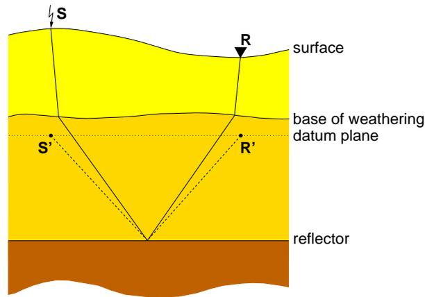
**Figure 1:** Raypath with a low velocity layer. Redatuming achieved by field static correction substitutes the surface by a datum plane beneath the low velocity layer, i. e., source S and receiver R are moved to S' and R' on the datum plane, respectively.
