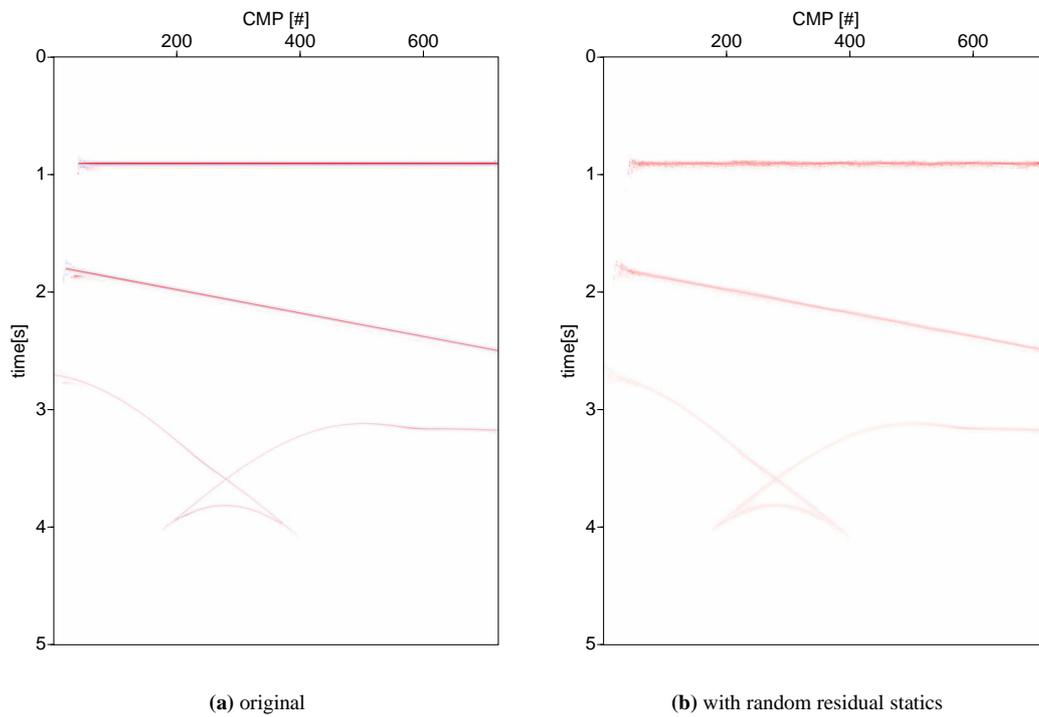
**Figure 6:** Simulated ZO section of the optimized 2D ZO CRS stack from a) the original synthetic data set and b) with random residual statics added.
