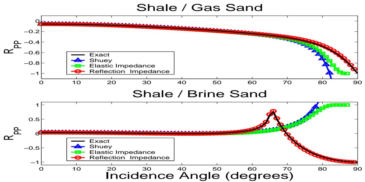
**Figure 2:** P-P reflection coefficient for Class II model given in Table 1: shale over gas sand (top) and shale over brine sand (bottom).
