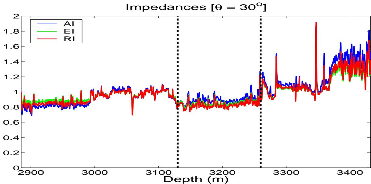
**Figure 5:** Comparison of the  $AI$  curve with the  $30^\circ EI$  and  $RI$  curves for the well log data given in Figure 4. The values were normalized so that at the first simple  $AI = EI = RI = 1$ .
