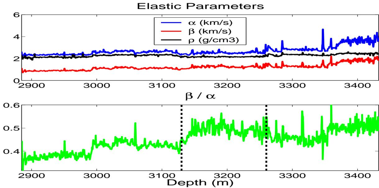
**Figure 4:** Well log data of an oil sand reservoir (dashed box) encased in marine shales.
