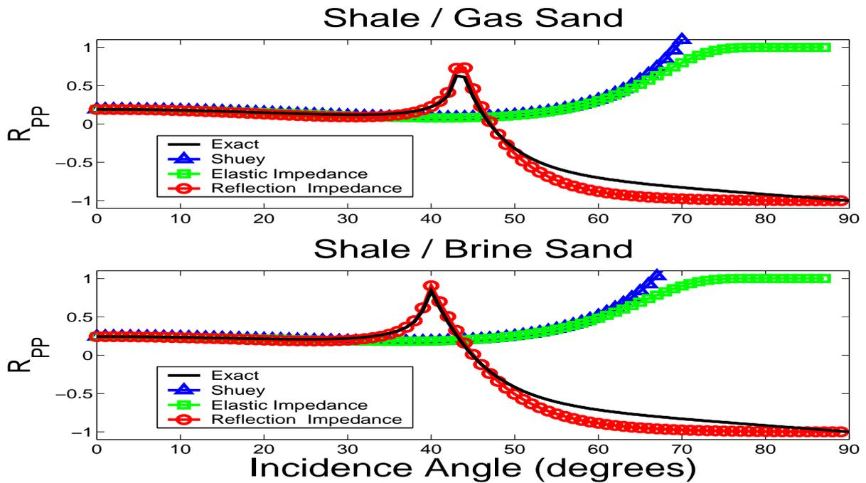
**Figure 1:** P-P reflection coefficient for Class I model given in Table 1: shale over gas sand (top) and shale over brine sand (bottom).
