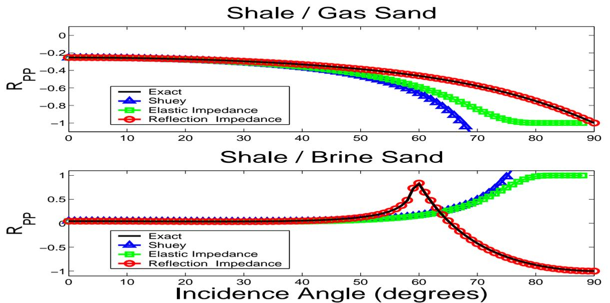
**Figure 3:** P-P reflection coefficient for Class III model given in Table 1: shale over gas sand (top) and shale over brine sand (bottom).
