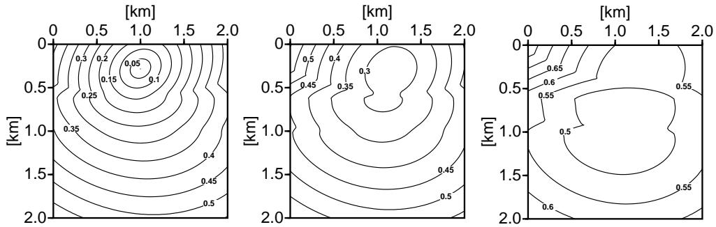
Figure 3: Wavefronts in a horizontally layered model;  $X - Z$ -slices with offset 0 km (left), 1 km (middle) and 1.3 km from the source.
