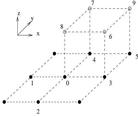
the ansatz used by (Ettrich, 1998) for the searched traveltime  $t_9$  at the corner point of a cubic cell is:
