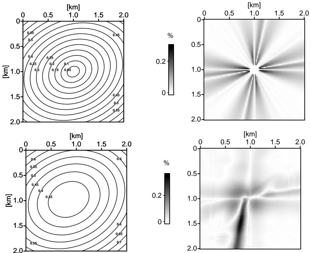
Figure 2: Wavefronts in a homogeneous elliptically anisotropic model:  $X - Z$ -slices with offset 0 km (upper, left) and 0.8 km (lower, left) from the source. The numerical solution is shown by solid lines, the analytical one is shown by dotted lines. On the right relative errors corresponding to the pictures on the left are given.
