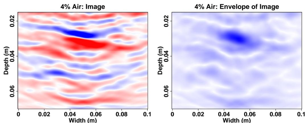
Figure 2: *The migration of the plane-wave response is on the left. On the right is the envelope of the migrated section.*
