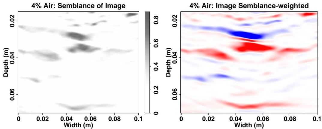
Figure 3: On the **left** the semblance is depicted which is calculated during the Kirchhoff migration. The **right** figure is the result of the migrated seismogram multiplied by the semblance section.
