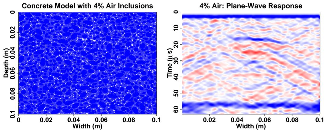
Figure 1: *On the left side is a heterogeneous concrete model with a defect, i.e. the crack. The ellipses represent gravel within cement. The right side shows the plane-wave response calculated with the Finite Difference program ULTIMOD using a rotated staggered grid.*
