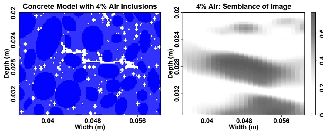
Figure 4: The **left** figure shows a zoom of the concrete and the **right** figure is the corresponding zoom of the semblance.
