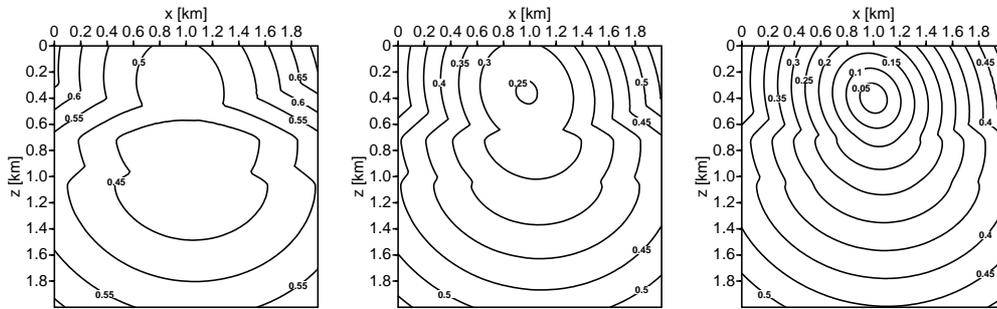
Figure 3: Wavefronts in a 3-D elliptically anisotropic inhomogeneous model;  $x$ - $z$ -slices with offset  $y=0$  km (left), 0.5 km (middle) and 1 km (right) from source.
