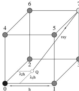
Figure 4: Cubical grid cell. Local straight ray segment reaching point 7 intersects boundary of cube in point  $Q$ .
