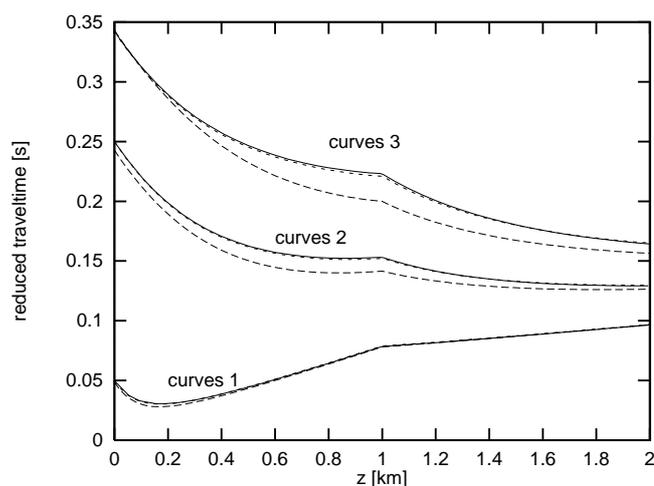
Figure 5: Curves of traveltime in an orthorhombic medium, computed with a ray tracer for anisotropic media (solid lines), and computed with the FD perturbation method (short dashes); reference traveltimes for the elliptically anisotropic reference medium (long dashes).
