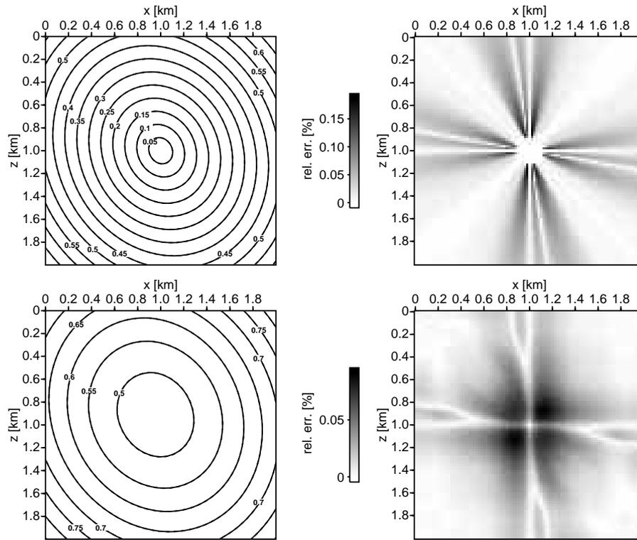
Figure 2: Left: Wavefronts in a homogeneous elliptically anisotropic model;  $x$ - $z$ -slices with offset  $y=0$  km (upper), and 1 km (lower) from source. Right: Corresponding relative errors.
