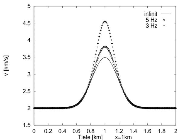
Figure 1: A vertical slice of the velocity function through the center of a Gaussian anomaly for three different frequencies computed by the perturbation scheme of Zhu.
