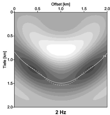
Figure 2: Snapshot at 0.42 s (gray scale plot); wavefront for a 2 Hz velocity smoothing (solid line) and high frequency wavefront (dashed line).
