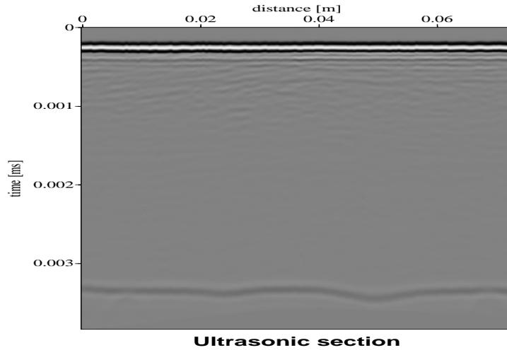
Figure 2: The early amplitude represents the input signal; the signal in the lower half of the section is the reflection at the bottom of the sample.
