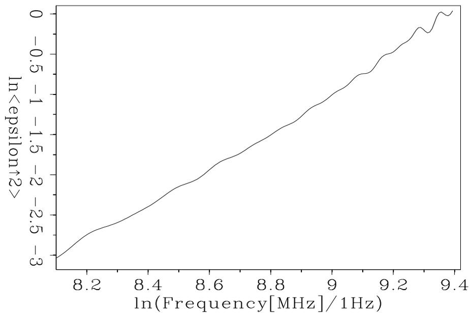
Figure 4:  $\ln\langle\epsilon^2\rangle - \ln\nu$  dependence for 1% strain; note the asymptotic behaviour toward a straight line.
