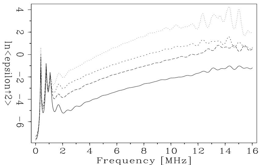
Figure 3:  $\ln\langle\epsilon^2\rangle$  - frequency dependence for different strains applied: 0% (solid), 1% (large dashed), 2% (fine dashed), 3% (dotted).
